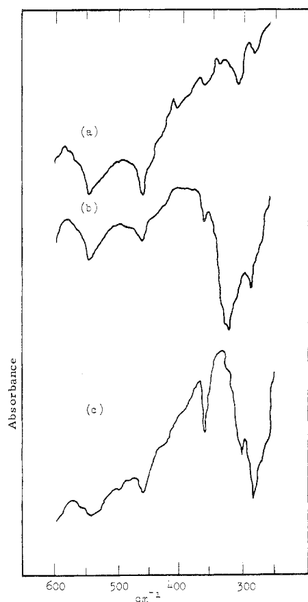
Figure 4. Far infrared spectra of (a) cis -[Rh(TTP)Br 2 ]Br, (b) [Rh(TTP)Cl] x Cl 2x , and (c) cis -[Rh(TTP)Cl 2 ]Cl.
